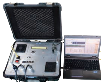
Safe Direction Drilling Panel (SDD)
