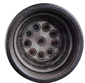
28-pin Male Plug (Use only 10 banana plugs)
